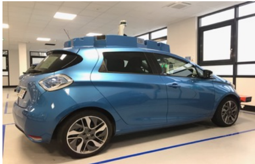
Data collection platform equipped with a VLP32C LIDAR
